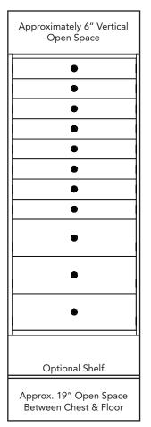
Not to Scale. Drawers can be placed higher or lower in the safe according to your preference. Custom configurations with different numbers and heights of drawers are available.
