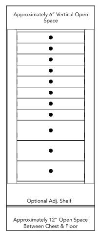
Not to Scale. Drawers can be placed higher or lower in the safe according to your preference. Custom configurations with different numbers and heights of drawers are available.
